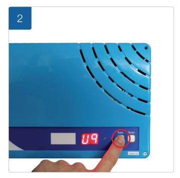
Press and hold the 'FUNC' button until the screen displays U9. Upon release at 'U9', the AlertMaxx2 will display 'C0'
