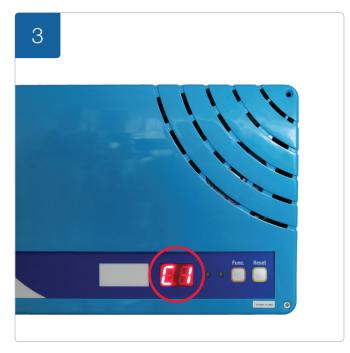
'C0' will automatically change to 'C1' to indicate the Wi-Fi configuration process has started.
