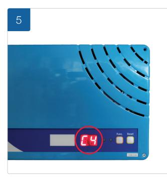
After connecting to WiFly, the AlertMaxx2 will show a 'C4' indicating you have successfully connected your device to the unit.
