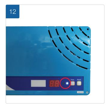
The AlertMaxx2 will flash the blue LED to indicate transmission of data and no code will be displayed on the screen.
