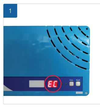
The AlertMaxx2 will show 'EC' when the unit has lost connection to the internet. Follow this guide if the Wi-Fi name, password or internet provider has changed.
