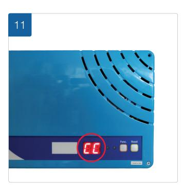
The AlertMaxx2 will now display 'CC' to indicate the configuration has been successful.
