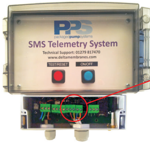
Connector blocks used for inputs from external devices
