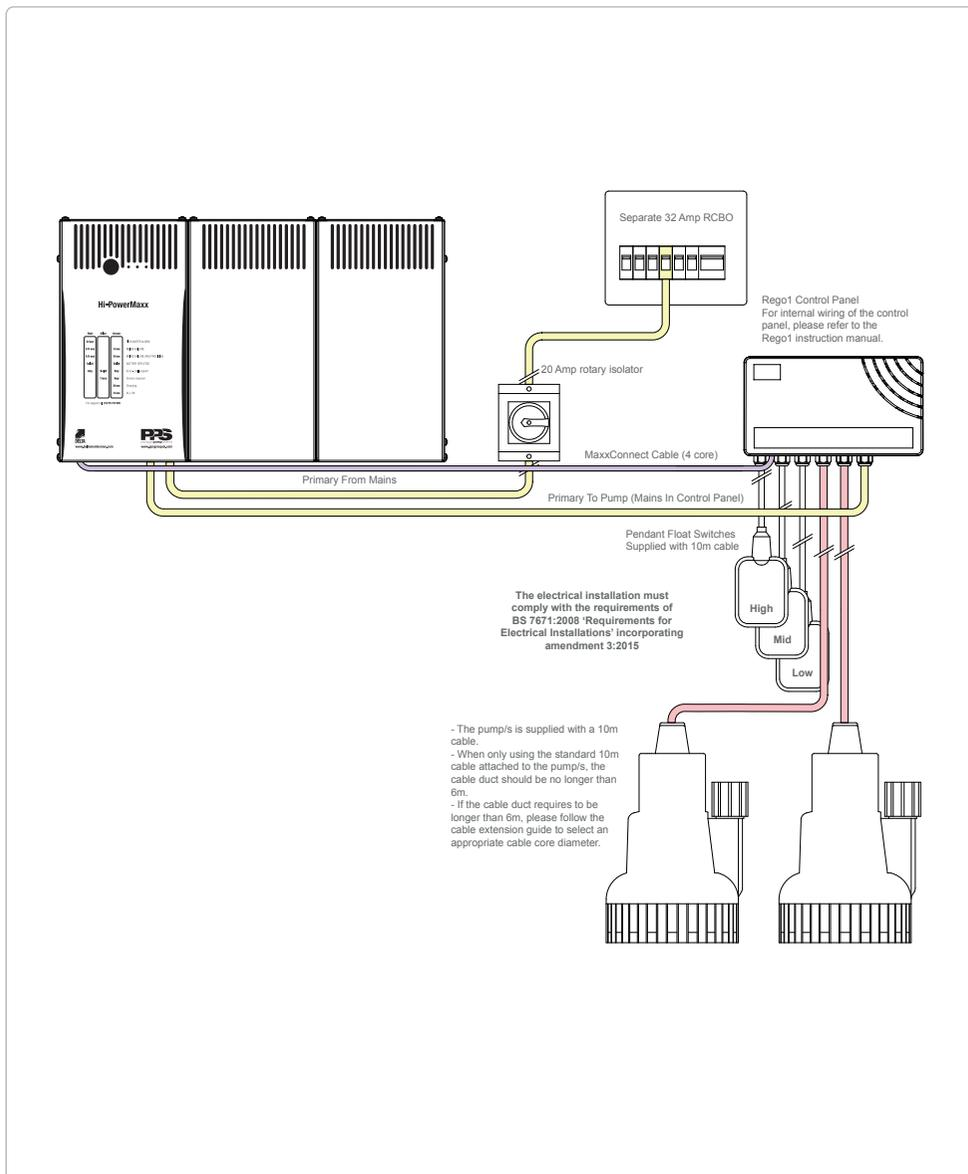
Figure 6. Rego1 typical wiring schematic (inc. battery backup)
