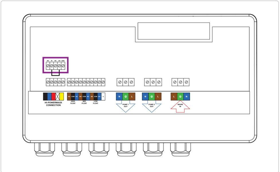
Figure 5. Typical Volt Free Relay (VFR) connection link
