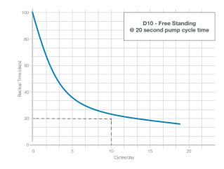
Mean average cycles/day = 10. Sample taken from 120 remote monitored ground water pump stations.
