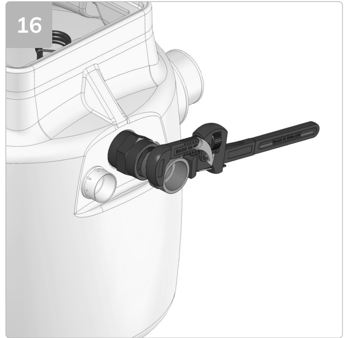
Screw the high pressure male iron into the female iron.
