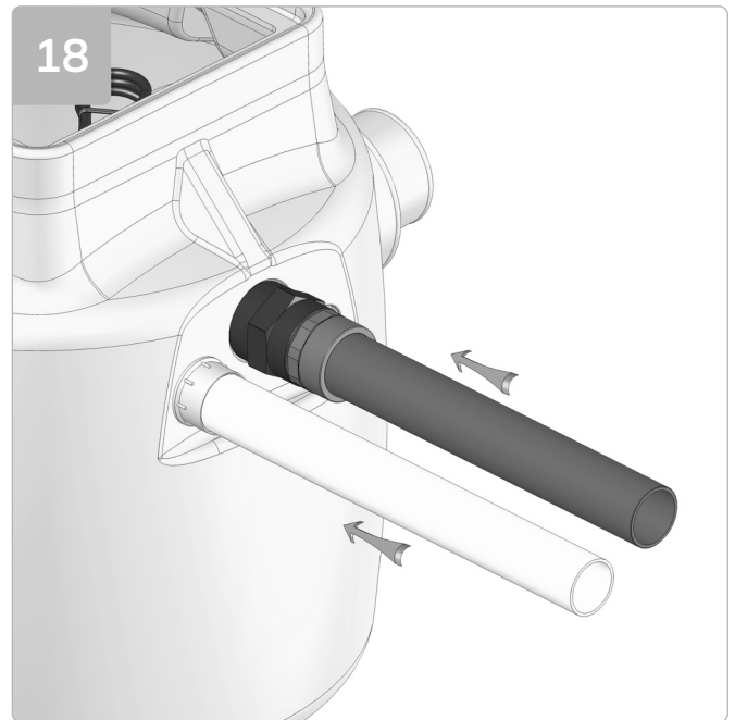
Push discharge and cable duct pipe into their respective male iron, twisting the pipe as it is pushed into the male iron to remove any trapped air.
