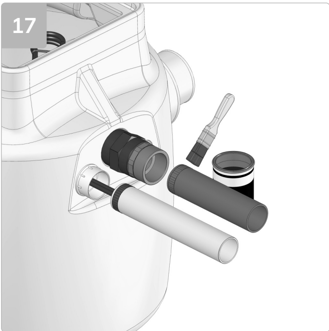
Apply high pressure glue around the first 20mm of the external face of the discharge and cable duct pipe and internal side of their respective male iron.
