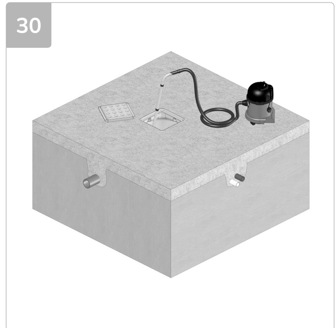
Manually remove any debris from chamber and residual water using a wet vac.
