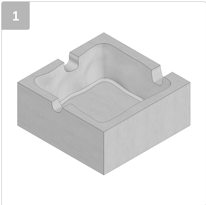
1 Excavate hole for chamber. Refer to section 10.0 for RC box internal dimensions.
