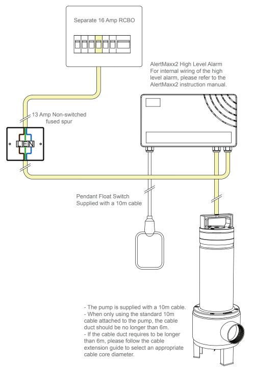
The electrical installation must comply with the requirements of BS 7671:2018 'Requirements for Electrical Installations' incorporating the latest amendment.
